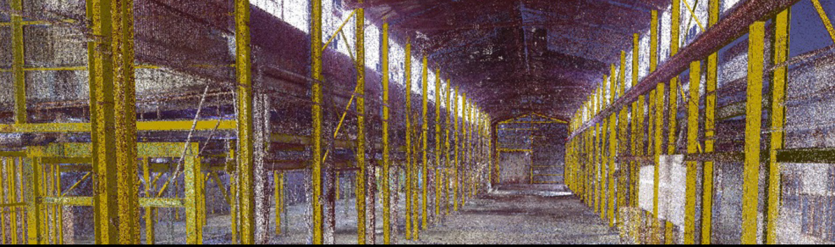
Registered laser scan point cloud of foundry interior, showing partially modeled steel columns & beams.
