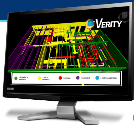
Verity's "stop light" variance classification gave Beck a quick overview of construction quality.
