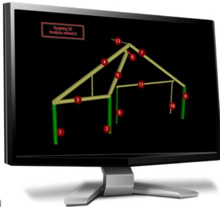
each individual beam to see if it deviated more than that distance from its designed position along the x, y or z axis. The software even checked for unplanned twists, bends and sags in the members.
